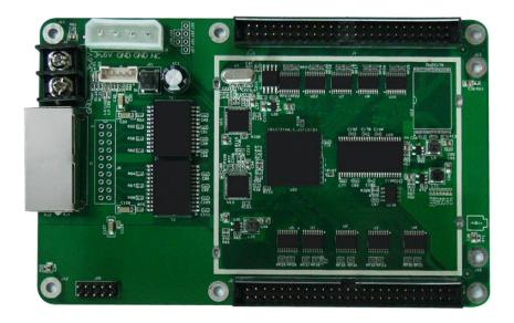
In addition to inherit all the advantages and features 5A had, i5A adopts a new generation of system architecture, and possesses more intelligent function and more stable system. i5A receiving card supports a range of more intelligent and high-end functions like program arbitrary switching, external connect to LCD display module, etc., which lead LED control system to a brand new level.
